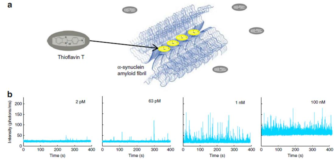
AttoBright is  $10^6$  times more sensitive than bulk measurement to detect  $\alpha$ Syn fibrils.
