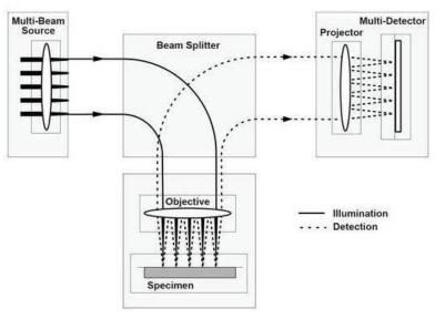
Schematic of the multi-beam microscope
