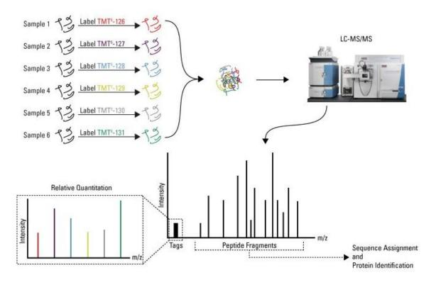
The combined M-F-N-R regions of the tags have the same total molecular weights and structure so that during chromatographic separation and in single MS mode, molecules labeled with different tags are indistinguishable.
